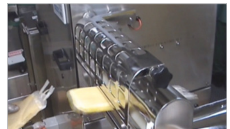
The squeeze roller in operation.
