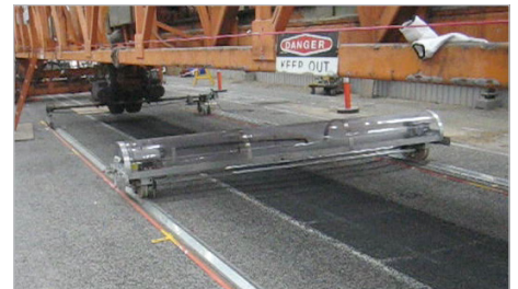
The Transverse Profiler installed at AARB underneath the ALF.
